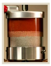
**Ultra Spacer**® can be weighted up to 19.0 ppg with barite or hematite.
